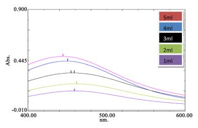
**Figure 2.** UV-visible spectrum of synthesized silver nanoparticles (AgNPs) using different volumes of the extracts (1 - 5 ml).
