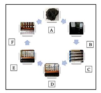
**Figure 1.** Biosynthesis of Silver nanoparticles. (A) Powder of *N. sativa* seeds; (B) homogenized suspension; (C) The extract after centrifugation; (D) Silver nitrate 1 M (10 ml); (E) & (F) The process of reduction after addition of the extract indicated by changing in color.
