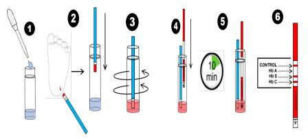
**Figure 1.** Procedure of the HemoTypeSC<sup>TM</sup> (From Manufacturer: Product # HT111, USA).
