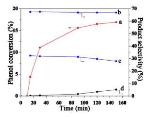
**Figure 3.** Effect of reaction time on the activity over Fe-BTC for phenol hydroxylation with phenol: $H_2O_2$  ratio of 1:1 at 50°C: (a) phenol conversion, (b) CAT selectivity, (c) HQ selectivity and (d) BQ selectivity.
