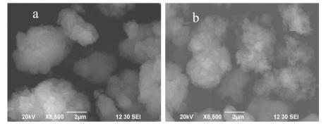
**Figure 5.** Scanning electron microscope of (a) fresh Fe-BTC and (b) reused Fe-BTC catalyst after fourth run. 20 kV accelerating voltage, the X8500 current magnification and 2  $\mu$ m scale bar were applied in this scanning.
