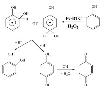
**Scheme 2.** Reaction path for phenol hydroxylation reaction catalyzed over Fe-BTC.
