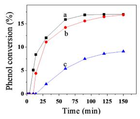
**Figure 2.** Effect of phenol to  $H_2O_2$  ratio for phenol hydroxylation at 50 °C: (a) 1:2, (b) 1:1 and (c) 1:0.5.
