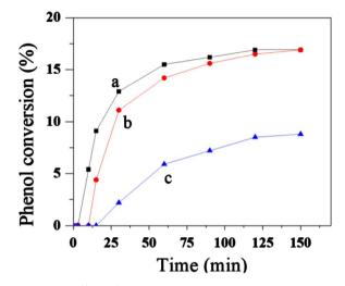
**Figure 1.** Effect of reaction temperature on the catalytic activity over Fe-BTC for phenol hydroxylation of phenol with phenol:  $H_2O_2$  ratio of 1:1: (a) 70°C, (b) 50°C and (c) 35°C.
