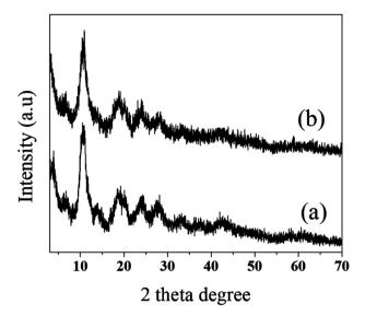
**Figure 4.** X-ray powder diffraction patterns of (a) Fe-BTC and (b) reused Fe-BTC catalyst after fourth run.
