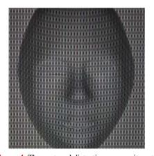
**Figure 4.** The captured distortion composite pattern modulated by height of the face model.
