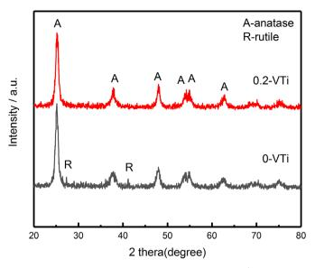
**Figure 2.** XRD patterns of the catalysts with various Ti<sup>3+</sup> doping.
