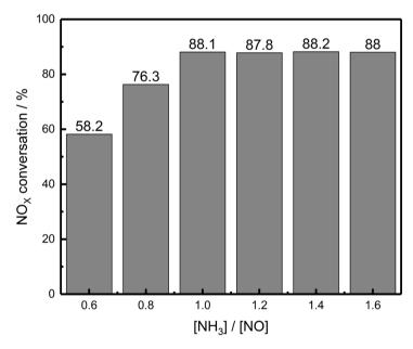
**Figure 6.** Effect of  $[NH_3]/[NO]$  molar ratio on catalytic activity at 210°C. Reaction conditions: [NO] = 500 ppm,  $O_2 = 5\%$ , GHSV = 23,885 h<sup>-1</sup>, balance N<sub>2</sub>, total flow rate 100 mL/min.
