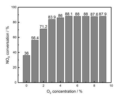
**Figure 5.** Effect of the  $O_2$  concentration on catalytic activity at 210°C. Reaction conditions: [NO] = [NH<sub>3</sub>] = 500 ppm, balance N<sub>2</sub>, GHSV = 23,885 h<sup>-1</sup>, total flow rate 100 mL/min.
