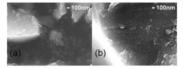
Figure 3. SEM micrographs of the 0.2-VTi catalyst, (a) fresh, (b) used.
