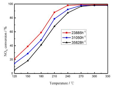
**Figure 7.** Effect of GHSV on catalytic activity. Reaction conditions: balance  $N_2$ , total flow rate are 23,885  $h^{-1}$ , 31,050  $h^{-1}$  and 35,828  $h^{-1}$  respectively.
