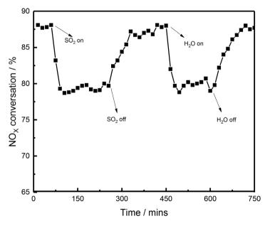
**Figure 9.** Effect of  $H_2O$  and  $SO_2$  on catalytic activity at 210°C. Reaction conditions: [NO] = 500 ppm,  $O_2 = 5\%$ ,  $SO_2 = 500$  ppm,  $H_2O = 5\%$ , GHSV = 23,885 h<sup>-1</sup>, balance N<sub>2</sub>, total flow rate 100 mL/min.
