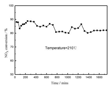
**Figure 8.** Effect of reaction time on catalytic activity at 210°C. Reaction conditions: [NO] = 500 ppm,  $O_2 = 5\%$ , GHSV = 23,885 h<sup>-1</sup>, balance N<sub>2</sub>, total flow rate 100 mL/min.
