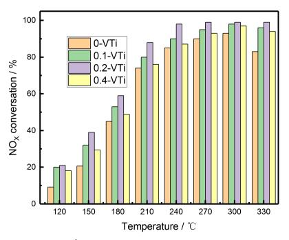
**Figure 1.** Effect of  $Ti^{3+}$  self-doped  $V_2O_5/TiO_2$  catalyst on  $NO_X$  conversation.
