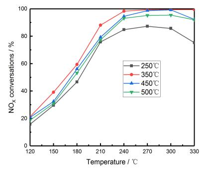
**Figure 4.** Effect of Ti<sup>3+</sup> catalysts of various calcined temperature of the support. Reaction conditions:  $[NO] = [NH_3] = 500$  ppm,  $O_2 = 5\%$ , balance  $N_2$ , GHSV = 23,885 h<sup>-1</sup>, total flow rate 100 mL/min.
