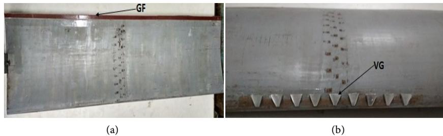
**Figure 3.** Aerofoil geometry with GF and VG. (a) Eppler with GF; (b) Eppler with VG.
