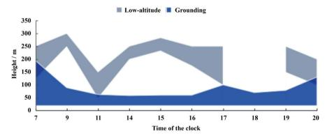
Figure 2. Low-altitude and grounding inversion height timing changes.
