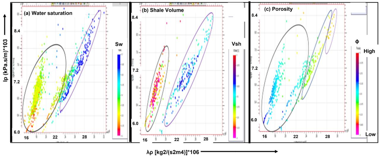
**Figure 8.** (a) (b) (c). Cross-plots of acoustic impedance ( $I_p$ ) versus Lambda-Rho ( $\lambda\rho$ ), color coded with water saturation, shale volume and porosity, respectively.
