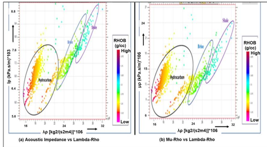
**Figure 6.** (a) (b). Cross-plots of rock attributes properties for sand 4 reservoir, color-coded with density.
