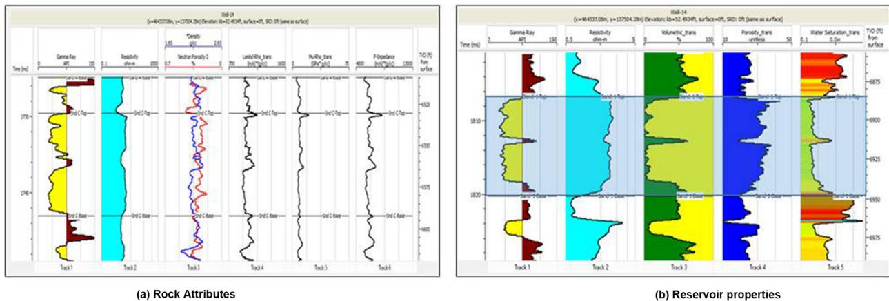
Figure 5. (a), (b). Modelled Pseudo-logs of elastic and reservoir properties for well 14.
