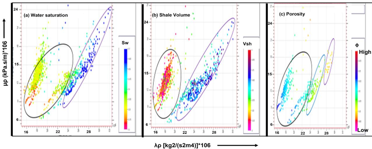
**Figure 7.** (a) (b) (c). Cross-plots of Mu-Rho ( $\mu\rho$ ) versus Lambda-Rho ( $\lambda\rho$ ), color coded with water saturation, shale volume and porosity, respectively.
