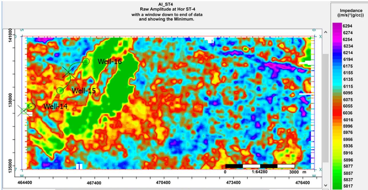
Figure 10. Acoustic impedance horizon map for H4.
