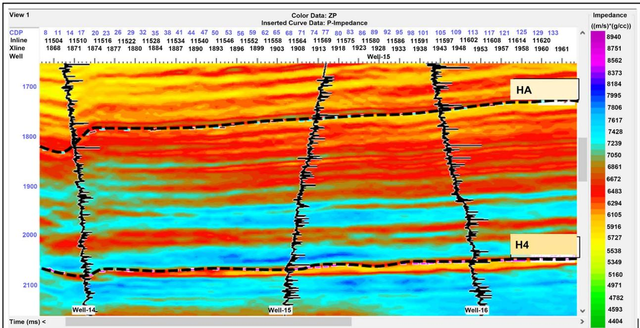
**Figure 9.** Cross section of acoustic impedance ( $I_p$ ).
