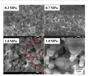
Figure 6. SEM images of combustion products synthesized at different N<sub>2</sub> pressures.
