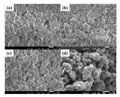
**Figure 7.** SEM images of sample M-3: (a) Center; (b) Intermediate; (c) Outside; (d) Magnification of (c).
