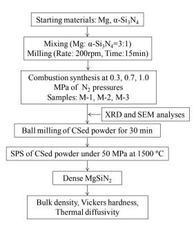
Figure 1. Flow chart of the experimental procedure for synthesizing MgSiN<sub>2</sub>.
