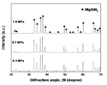
Figure 4. XRD patterns of combustion product synthesized at different N<sub>2</sub> pressures.
