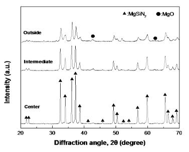
Figure 5. XRD patterns of the combustion product of sample M-2.
