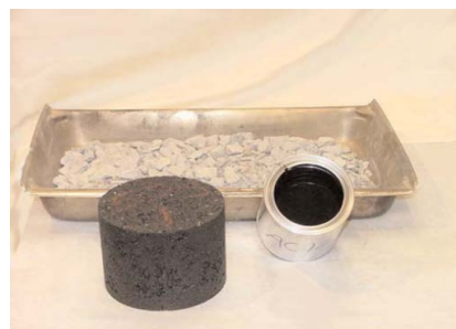
Figure 5. A compacted HMA laboratory specimen and the aggregate and asphalt used to prepare it.
