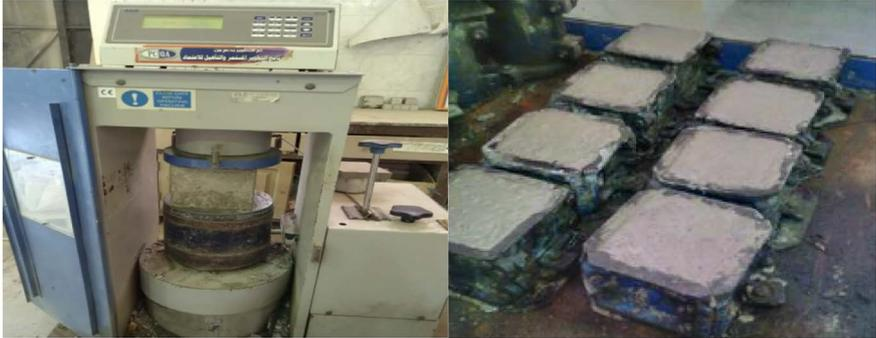
**Figure 7.** Casting and testing of cube specimens.
