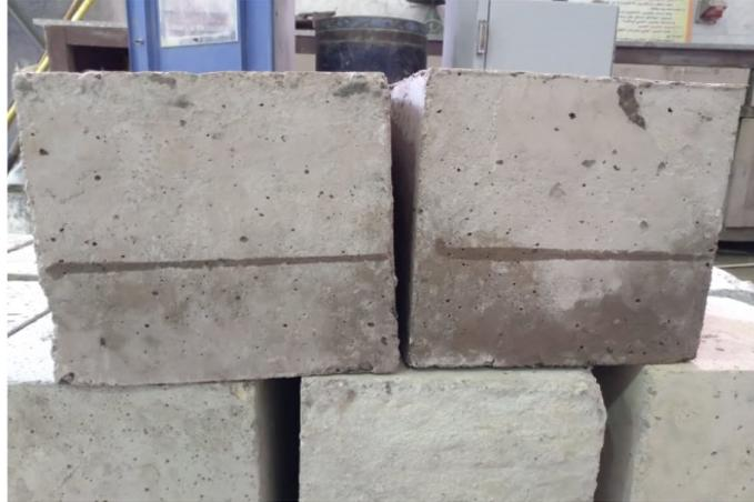
**Figure 17.** Permeability sample with different type of aggregate.
