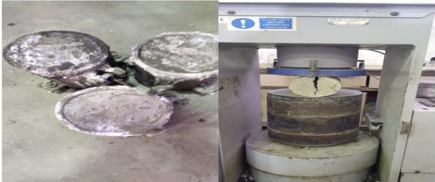
**Figure 8.** Casting and testing of cylinder specimens.
