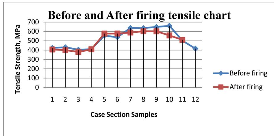
**Figure 13.** Tensile strength chart for samples before and after firing.
