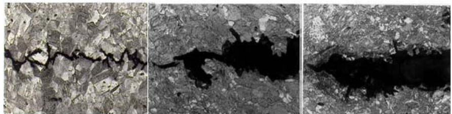
Figure 4. Intercrystalline feature cracks. Amplification = 250x; Etched in 10% ammonium persulphate [2].
