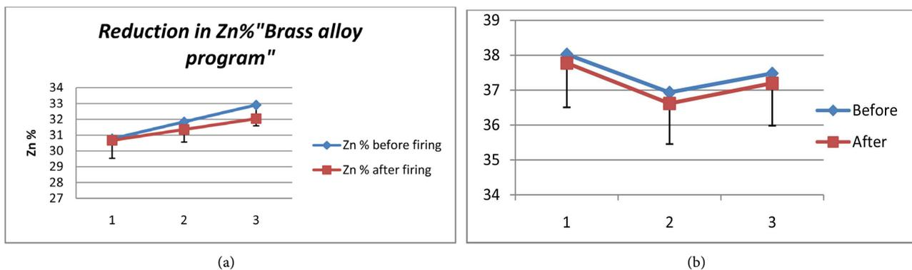
**Figure 11.** (a) Reduction in Z% by “brass alloy program”; (b) Reduction in Z% by “brass high alloy program”.
