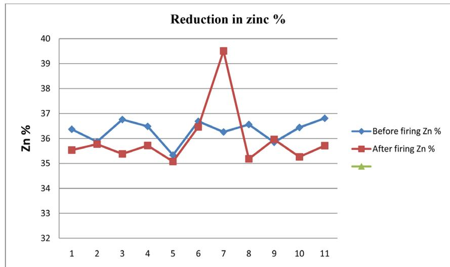
**Figure 12.** Reduction in Zn % before and after firing “High alloyed Brass program”.
