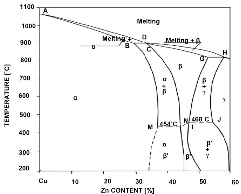
**Figure 1.** Binary diagram copper-zinc [1].
