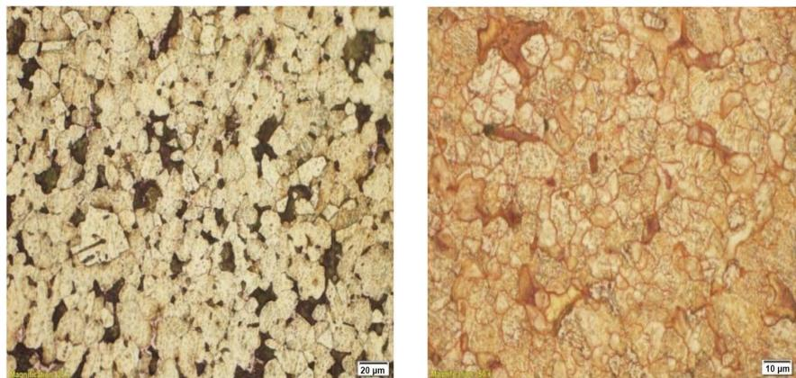
**Figure 7.** Structure before firing, left and after firing, right.
