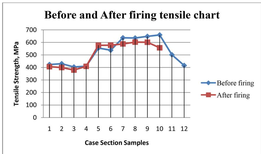
**Figure 9.** Tensile strength chart for samples before and after firing.
