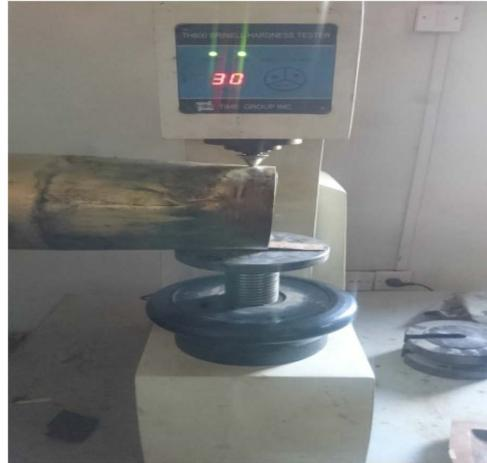
**Figure 5.** TH600 Brinell hardness test device with the sample mounted.
