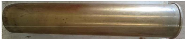
Figure 3. Typical fired brass cartridge case.
