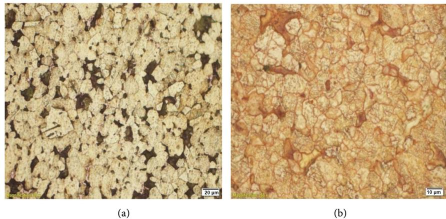
**Figure 14.** (a) microstructure before firing; (b) microstructure after firing.
