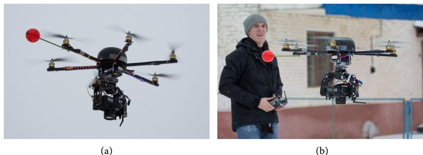
**Figure 1.** Helicopter-type UAV: (a) The UAV during the flight with a camera mounted in the gimbal; (b) The operator with the remote control of the UAV on the background.
