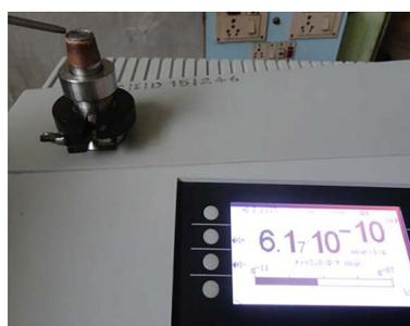
**Figure 6.** Helium leak test using MSLD.
