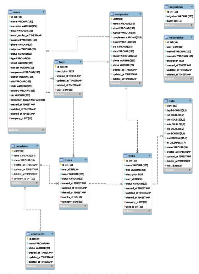
Figure 6. Entity Relationship Diagram (ERD) with the system database details.
