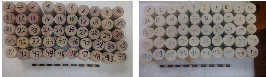
**Figure 23.** Preparation of the samples for mechanical testing and ultrasonic testing.
