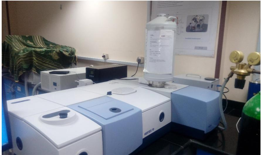
**Figure 9.** FT Raman Spectroscopy which have been used to identify the presence of certain functional groups in inorganic molecule.
