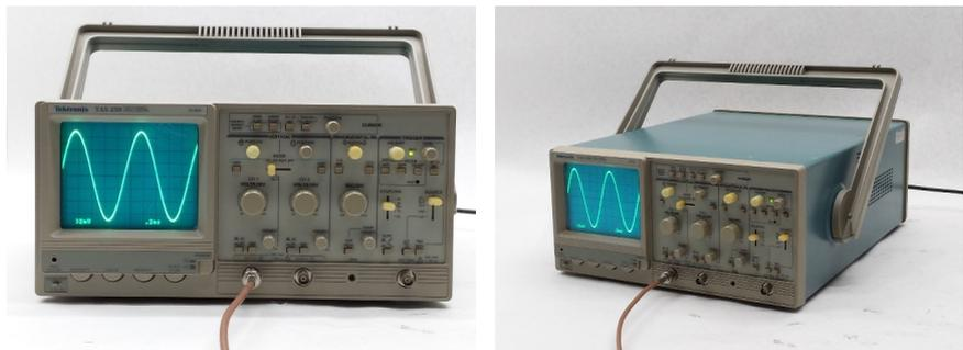
**Figure 18.** Tektronix TAS250 Digital Oscilloscope (seismic analyzer). The instrument which used for identification of seismic waves for the stone samples, this test carried out at faculty of science, geophysics department, Cairo University.
