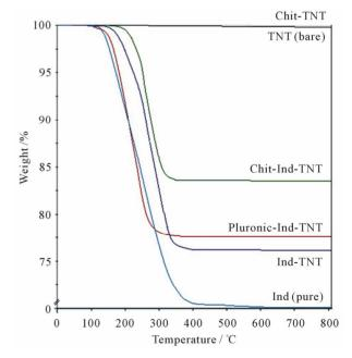
Figure 5. TGA graphs showing the amount of weight loss for drug and drug-micelle samples from bare and coated titania nanotube (TNT) arrays.
