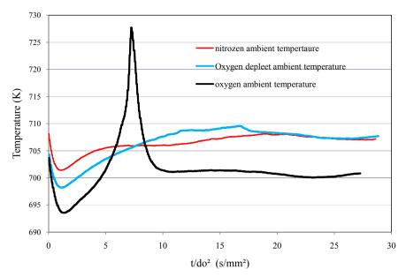
**Figure 8.** Effect of atmospheric oxygen on temperature viscinty the droplet evolution at ambient temperature of 703 K.
