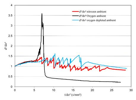
**Figure 7.** Effect of atmospheric oxygen on puffing and Bursting phenomena at ambient temperature of 703 K.
