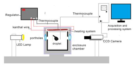
Figure 1. Schematic diagram of experimental setup.
