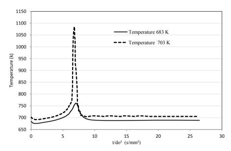
**Figure 6.** Evolution of temperature curve in the vicinty of droplet versus normalized time at 683 K and 703 K.
