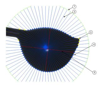
**Figure 2.** Projected surface determination of the droplet during the vaporization process. 1: Search box, 2: Edge detection Line, 3: Edge detected, 4: The edge used in the calculation of the ellipse, 5: Axes of the calculated ellipse.
