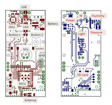
Figure 3. Double Sided PCB for V3 board.
