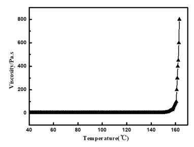
Figure 3. Viscosity vs temperature for BSA resin.
