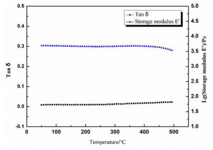
Figure 6. DMA curve of cured BSA.
