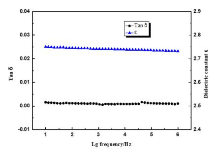
Figure 5. Dielectric curve of cured BSA resin.
