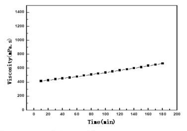
Figure 4. Viscosity of BSA resin at different time.
