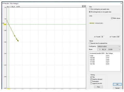
Figure 5. Maximum additional power transfer at 0.9 pu in PV curve.
