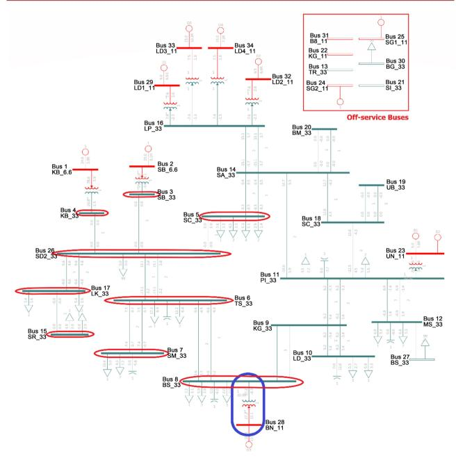
Figure 3. N-1-1 case with affected buses when outage of transformer branch from bus 8 to bus 28.
