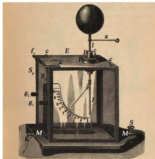
**Figure 2.** Kolbe electrometer, a precision form of gold leaf instrument. This has a light pivoted aluminium vane hanging next to a vertical metal plate. When charged the vane is repelled by the plate and hangs at an angle. However, also it is possibly affected by the Ampere forces, which usually cannot become apparent, due to the relatively low magnitude of the Ampere forces compared to the masking Coulomb forces.
