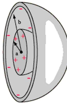
Figure 3. Two concentric spheres forming a spherical capacitor.
