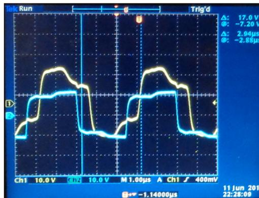
One important picture showing practically no anisotropy and no gain of energy of the same identical height ac pulses (Triangles on the left, indicate the zero point line of the two graphs respectively), departing and returning-for a short loop of 0.7 meters, unlike the long 134 meters loop.
