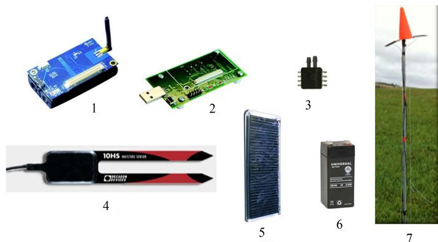
**Figure 2.** IRIS Mote XM2110CA (1) gateway unit MIB510CA (2) pressure sensor. “Freescale” MPXV7007DP (3) soil moisture sensor (E240-40761) 10HS (4) 6V DC 100 mA solar panel (5) 4.0 V (4.5 Ah) lead-acid battery (6) assembly of a node in the field (7).
