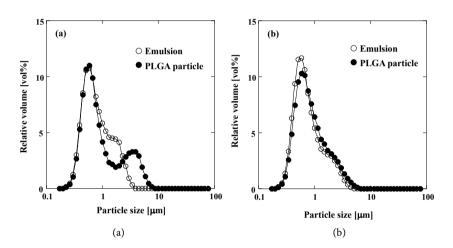
**Figure 2.** Size distribution of emulsions before the solvent evaporation process and prepared PLGA particles. Emulsion type used in particle preparation: (a) W/O/W emulsion; (b) S/O/W emulsion.
