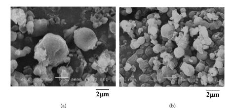
**Figure 1.** SEM images of the particles prepared using (a) W/O/W emulsions and (b) S/O/W emulsions.
