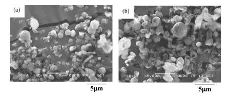
**Figure 3.** SEM images of the particles with the different content of lipophilic surfactant. (a) 3 wt%, (b) 10 wt%.
