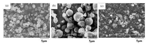
**Figure 4.** SEM images of the particles prepared with the emulsions containing different hydrophilic surfactants. Surfactant: (a) PVA; (b) L-1695; (c) Cholic acid.
