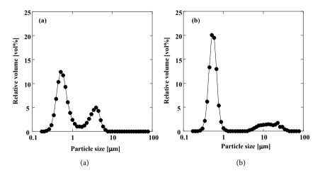
**Figure 5.** Size distribution of the particles controlled by membrane emulsification. Hydrophilic surfactant: (a) PVA; (b) Cholic acid.
