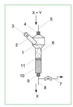
**Figure 2.** The sketch of mechanochemical sorption apparatus; 1—sorption column, 2—disintegrator, 3—actuator, 4—filter, 5—inlet pipe, 6—Me particles, 7—sampling line, 8—gas outlet, 9—filter, 10—pile of waste MeY, 11—layer of reacting powder.
