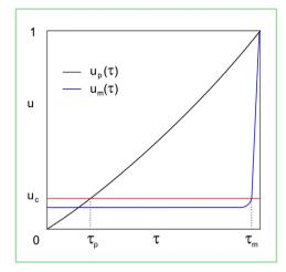
**Figure 5.** The dependence of the dimensionless impurity concentration in the outlet gas on the process time;  $u_p(\tau)$ —impurity concentration in the outlet of the gas purifier,  $u_m(\tau)$ —the impurity concentration at the outlet of the mechanochemical apparatus,  $\tau_p$  and  $\tau_m$ —the working time of the gas purifier and the mechanochemical apparatuses correspondingly,  $u_c$ —see  $u_c$  in **Figure 1**.
