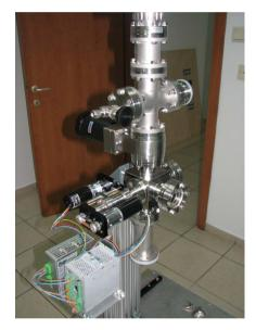
**Figure 3.** Laboratory scale mechanochemical sorption apparatus.
