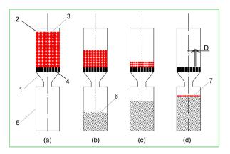
**Figure 7.** Schematic presentation of changes in the charge of sorption reactor with time. (a)—start, (b) and (c)—intermediate stages, (d)—final stage; 1—sorption column, 2—reactor, 3—particles of reactant Me, 4—dividing mesh, 5—waste collector, 6—MeY particles, 7—residual Me particles with the size of smaller than the separator mesh.
