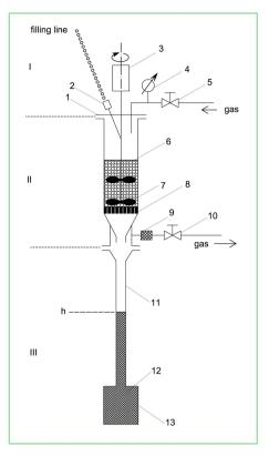
**Figure 6.** The sketch of reactive sorber. I—sorber head, II—high pressure reactor, III—bottom chamber; 1—flange, 2—charging port, 3—actuator of the magnetic stirrer, 4—manometer, 5—valve, 6—reactant, 7 stirrer blades, 8—dividing mesh, 9—filter, 10—valve, 11—connecting tube, 12—waste, 13—waste collector; h is the height of the accumulated waste.
