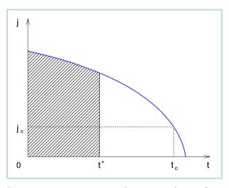
**Figure 8.** Gas capturing rate *j* in the reactive sorber as a function of time *t*.  $j_c$ —critical rate below which the gas quality becomes unsatisfactory,  $t^*$ —running time,  $t_c$ —time of safe operation of the sorber.
