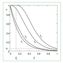
**Figure 1.** The distribution of impurity concentration in the gas phase along the sorption column at different moments of time. Here, *u* is dimensionless impurity concentration,  $\xi$  is dimensionless longitudinal coordinate,  $\tau$  is dimensionless time,  $\xi_c$  is the boundary of the exhausted powder, and  $u_c$  stands for the maximal allowed impurity concentration in the outlet gas.
