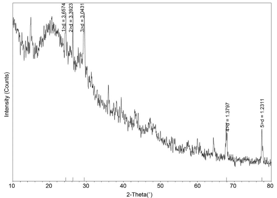
**Figure 4.** X-ray powder diffraction of burned SSC.
