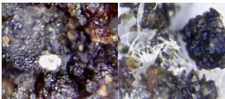
**Figure 5.** Microscopic photograph of the burned SSC (400× Digital Zoom).
