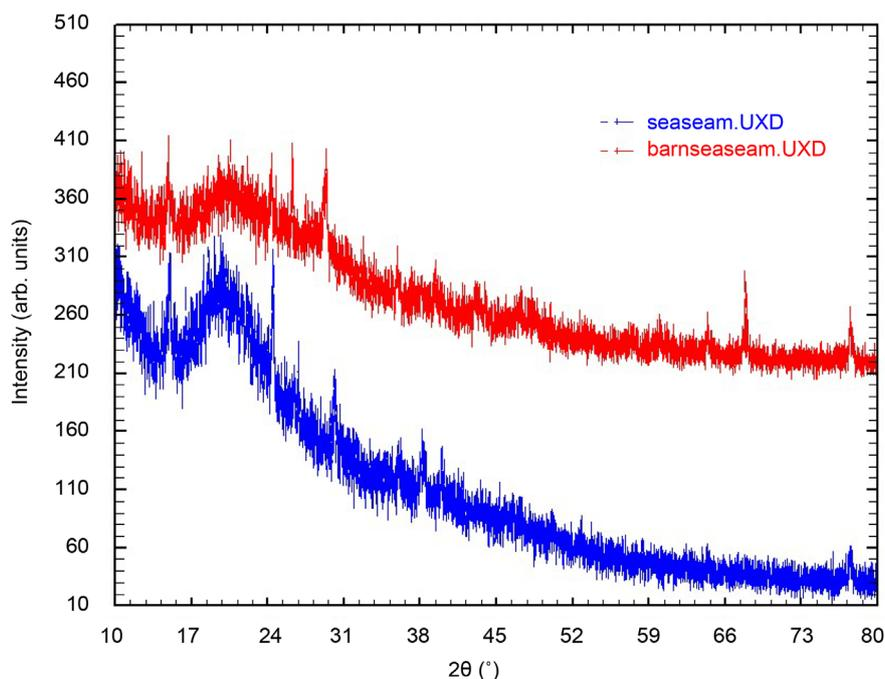
**Figure 2.** X-ray powder diffraction patterns of 1-nature, 2-burned SSC sample.
