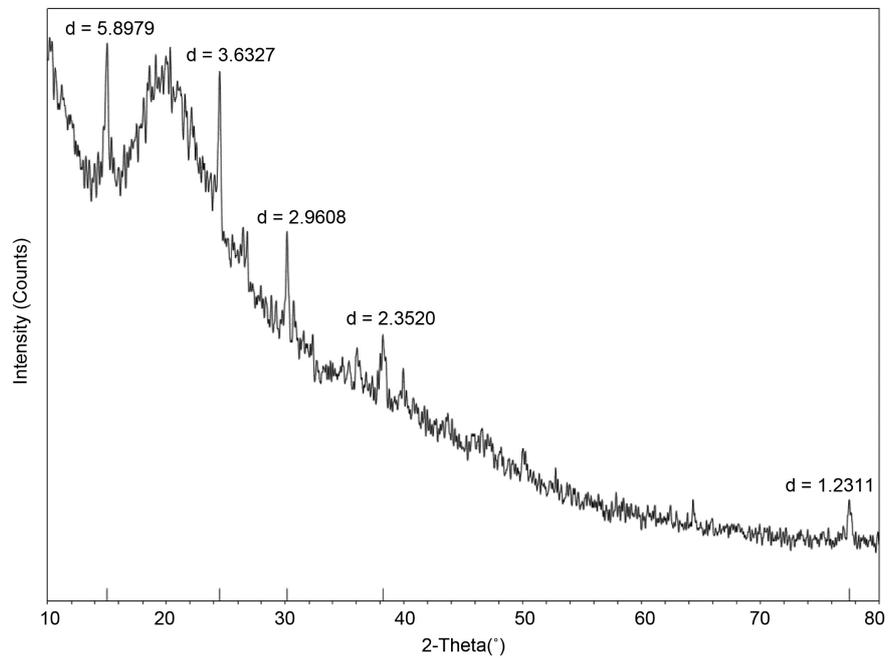
**Figure 3.** X-ray powder diffraction of nature SSC.
