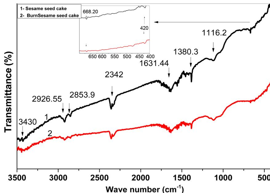
**Figure 6.** FTIR transmittance of SSC samples before and after burning process.
