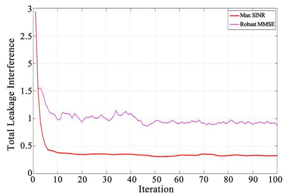
**Figure 2.** Sum of fraction of interference leakage to received signal at each user.  $M = N = 3$ ,  $D = 1$ ,  $K = 4$  interference network with  $\sigma^2 = 0.1$ , and  $\frac{P}{N_0} = 10$  dB.
