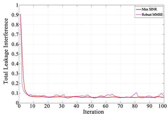
**Figure 3.** Sum of fraction of interference leakage to received signal at each user.  $M = 3$ ,  $N = 4$ ,  $D = 2$ ,  $K = 2$  interference network with  $\sigma^2 = 0.1$ , and  $\frac{P}{N_0} = 10$  dB.
