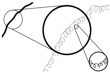
**Figure 1.** The same trajectory in space of a charged particle in an e.m. field observed with three different resolutions. At first sight each curve can be understood as the particle's trajectory but it could also not be.
