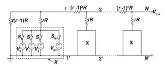
Figure 7. Digital to analog voltage converter.
