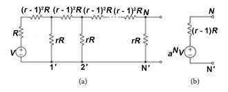
Figure 4. (a) Cascaded *n*-sections, (b) Thevenin equivalent circuit.
