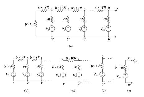
**Figure 6.** (a) Ladder with voltage sources, (b)-(e) circuits after applying successively Thevenin theorem.
