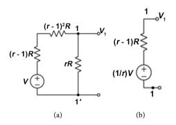
**Figure 2.** Scaled circuit of **Figure 1(b)** and its Thevenin equivalent.
