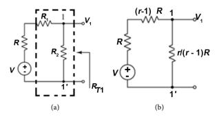
**Figure 1.** (a) A simplest possible attenuator; (b) Attenuator with values.
