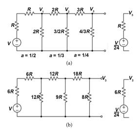
**Figure 5.** (a) 3 cascaded sections with different AFs; (b) Circuit after scaling with a factor of 6.
