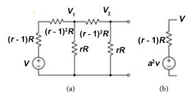
Figure 3. (a) Cascaded 2 sections, (b) Thevenin equivalent circuit.
