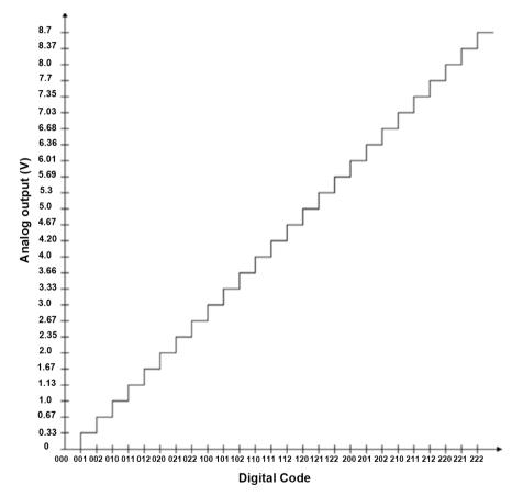
Figure 9. Plot of analog voltage output versus digital input.
