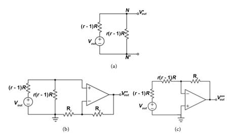
**Figure 8.** (a) Circuit with additional resistance connected; (b) Circuit with non-inverting amplifier; (c) Circuit with inverting amplifier.
