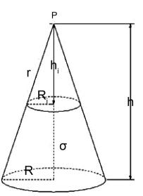
Figure 5. A conical uniform charge body.
