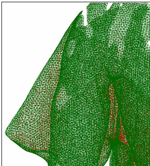
**Figure 10.** FEA mesh that shows irregular patches.
