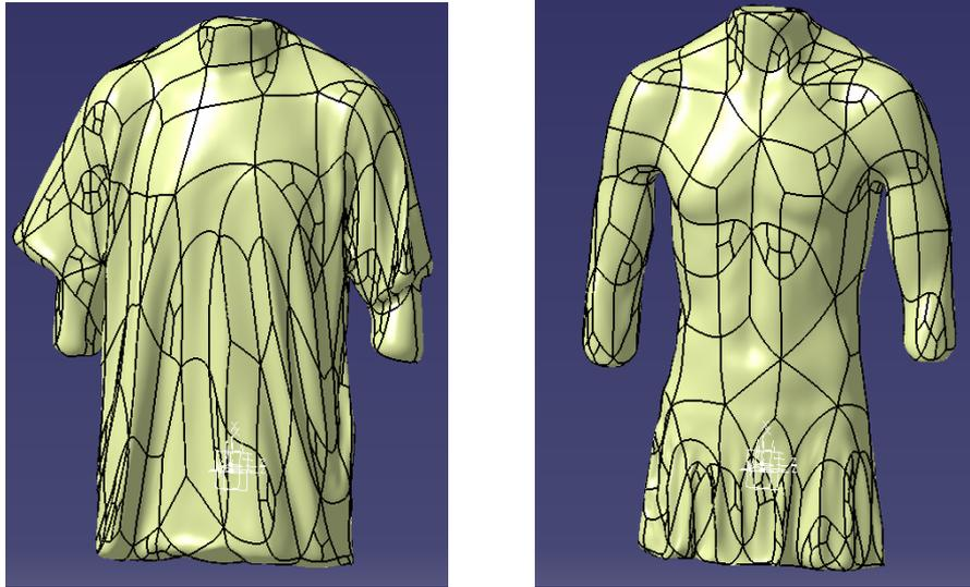
Figure 8. Surfaces created from clean mesh.
