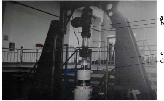
**Figure 3.** Bench test of the characteristics of hydro-pneumatic suspension: a—hydraulic cylinder, b—accumulator, c—test bench, d—hydraulic actuator.
