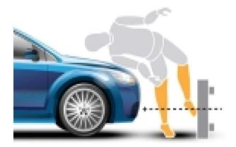
Figure 2. Schematic image of legform impacte test.
