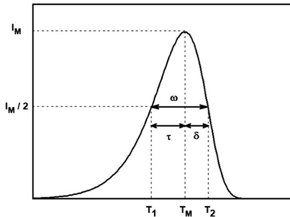
**Figure 3.** The geometrical parameters characterizing an isolated peak.
