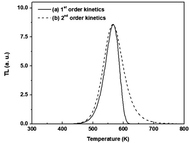
**Figure 2.** Variation of glow peak shape according to the kinetic process.
