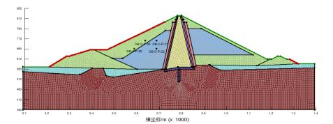
Figure 5. Finite element model of Nuozhadu core rockfill dam.
