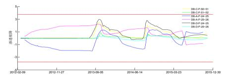
**Figure 4.** Curves of the measured seepage gradients between adjacent monitoring points in 780m height of core wall.
