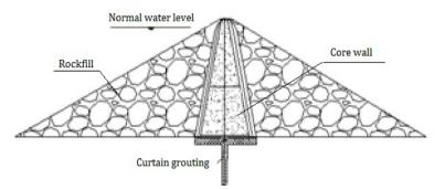
Figure 2. Structure of high core rockfill dam.
