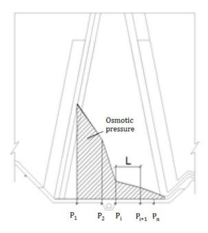
Figure 3. Layout of pressure gauges in core wall.
