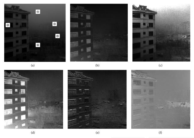
**Figure 3.** The multi optical parametric imaging effect under the fog. (a) The intensity figure; (b) Polarized radiation figure; (c) non-polarization radiation figure; (d) Linear polarization figure; (e) Circular polarization figure; (f) The polarization Angle of figure.
