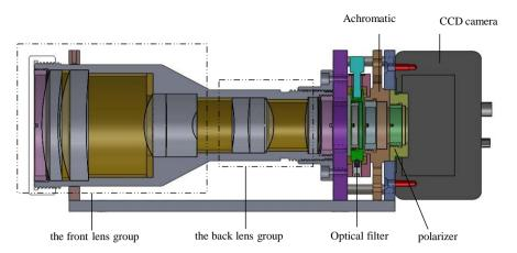
Figure 1. The multi optical parameter imaging system.
