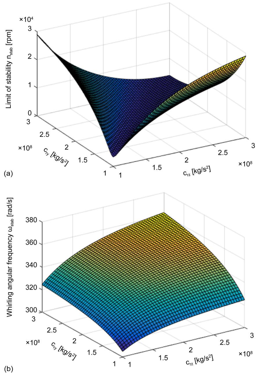
**Figure 10.** Influence of the bearing stiffness on (a) the limit of stability  $n_{stab}$  and on (b) the whirling angular frequency  $\omega_{stab}$  for a rigid foundation.
