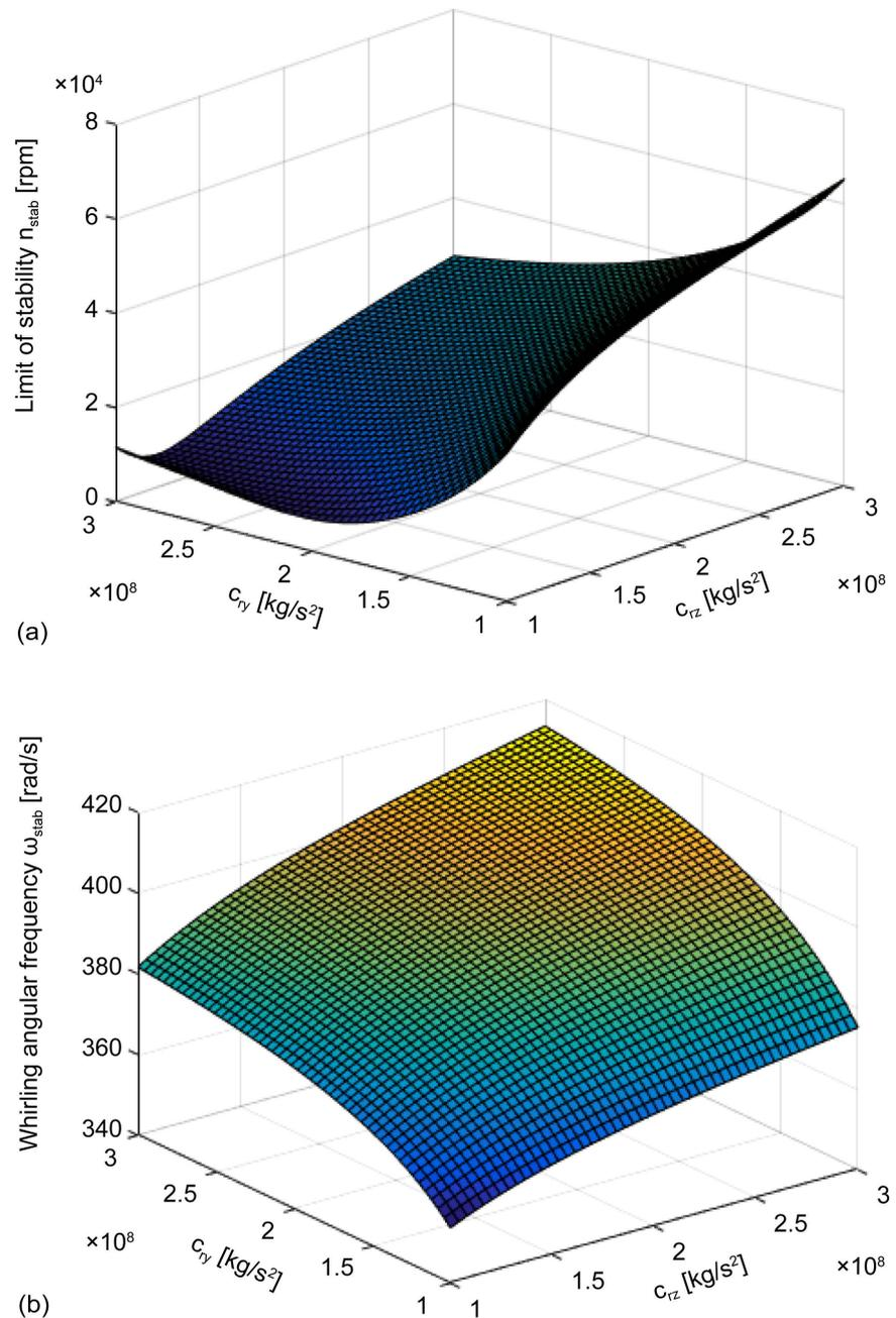
**Figure 8.** Influence of the bearing stiffness on (a) the limit of stability  $n_{stab}$  and on (b) the whirling angular frequency  $\omega_{stab}$  for the rated soft foundation (Table 1).
