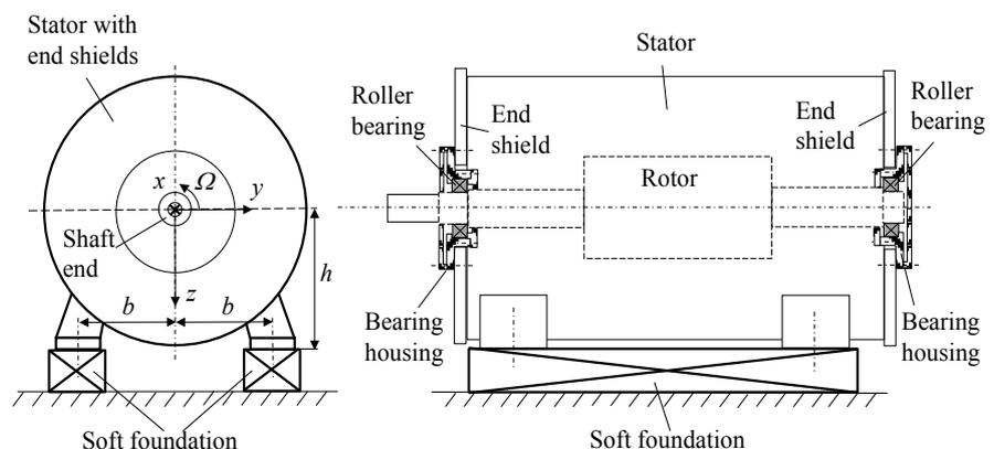
**Figure 1.** Special kind of rotating machine with rotor, roller bearings, bearing housings, end-shields and stator, mounted on a soft foundation.
