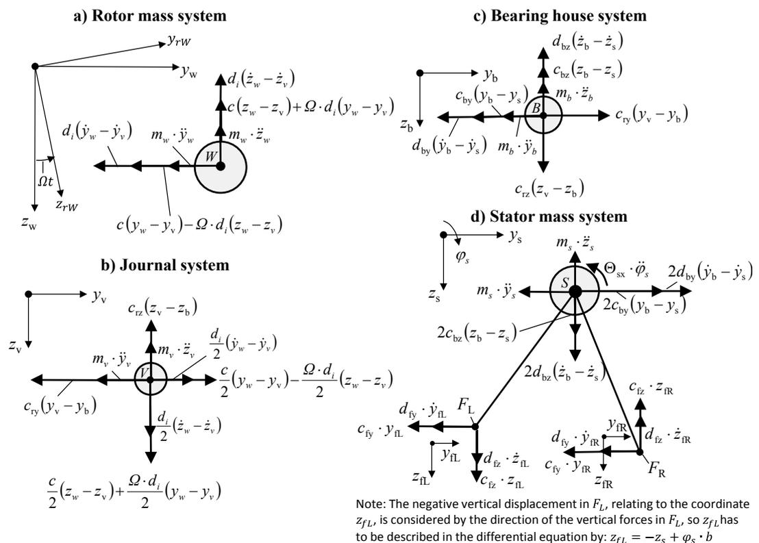
Figure 3. Vibration system cut free into subsystems.
