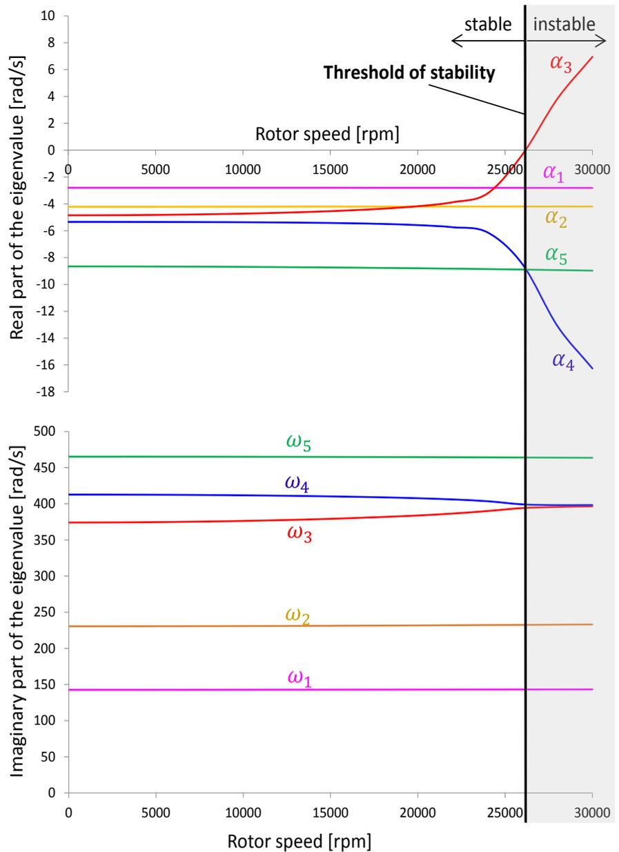
**Figure 5.** Eigenvalues, depending on the rotor speed and threshold of stability.
