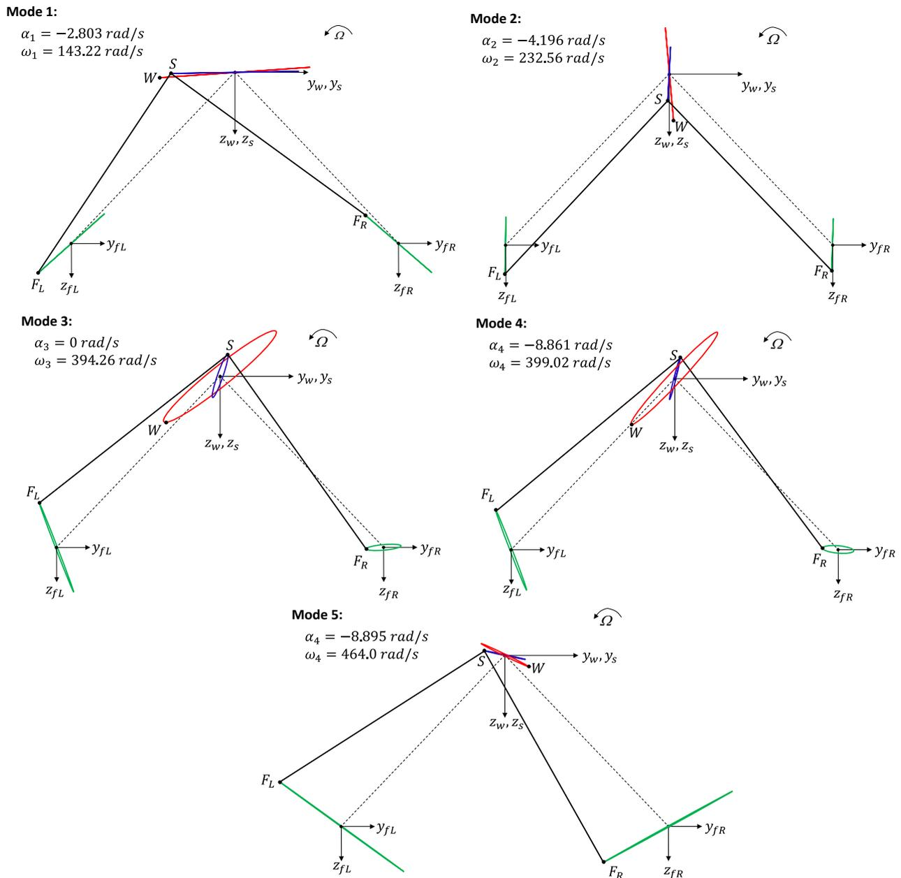
**Figure 6.** Mode shapes at the threshold of stability with  $n_{stab} = 26130$  rpm.
