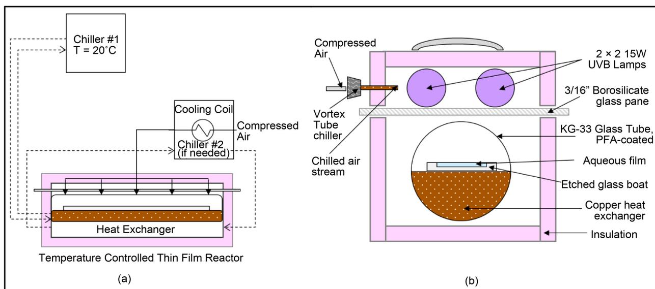
**Figure 1.** (a) Sketch of the thin film reactor assembly used in photo-oxidation experiments that test the effect of film thickness. Dashed lines represent coolant flow. (b) Cross-section of the thin film reactor [14].
