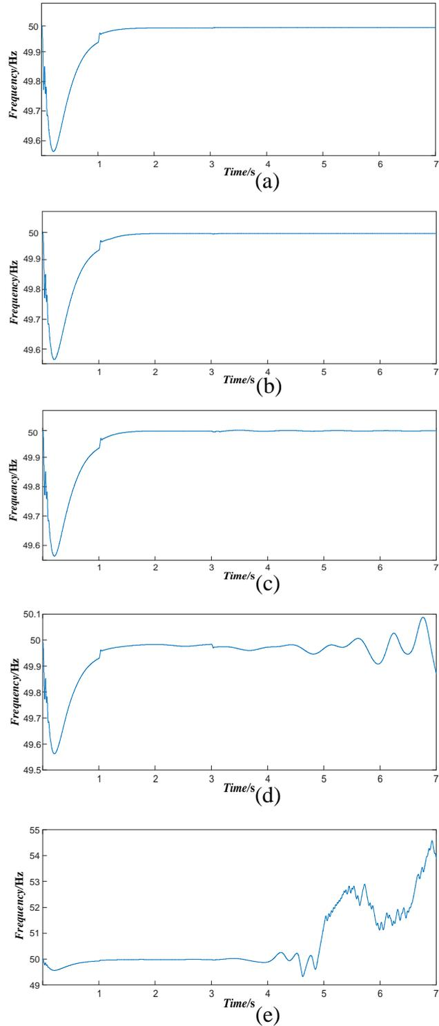
**Figure 7.** Waveform of frequency, (a)  $\tau = 0$ , (b)  $\tau = 0.1$  s, (c)  $\tau = 0.2$  s, (d)  $\tau = 0.3$  s, (e)  $\tau = 0.5$  s.
