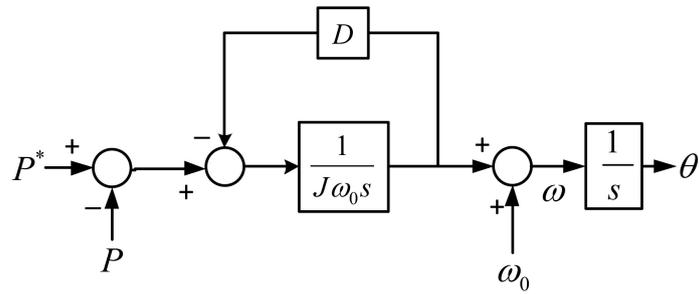
Figure 2. Active power-frequency droop controller.
