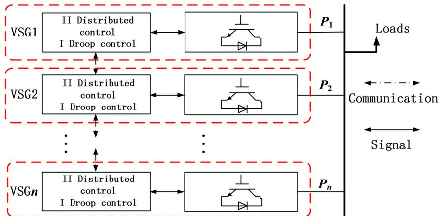
Figure 4. Coordinated control structure of VSGs.
