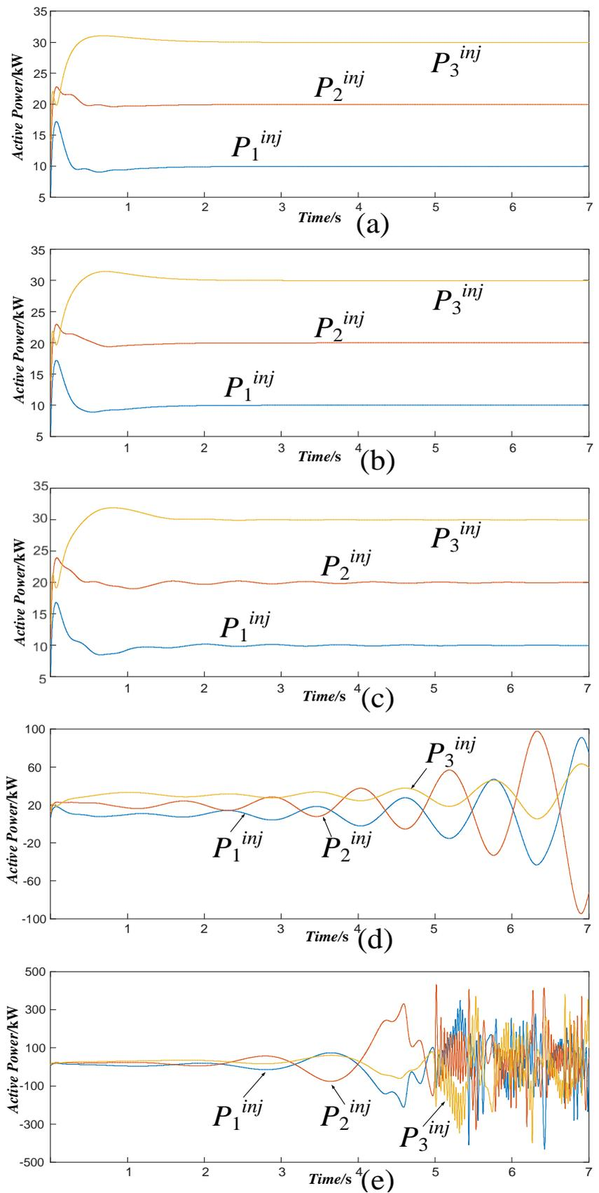
**Figure 8.** Waveform of active power, (a)  $\tau = 0$ , (b)  $\tau = 0.1$  s, (c)  $\tau = 0.2$  s, (d)  $\tau = 0.3$  s, (e)  $\tau = 0.5$  s.
