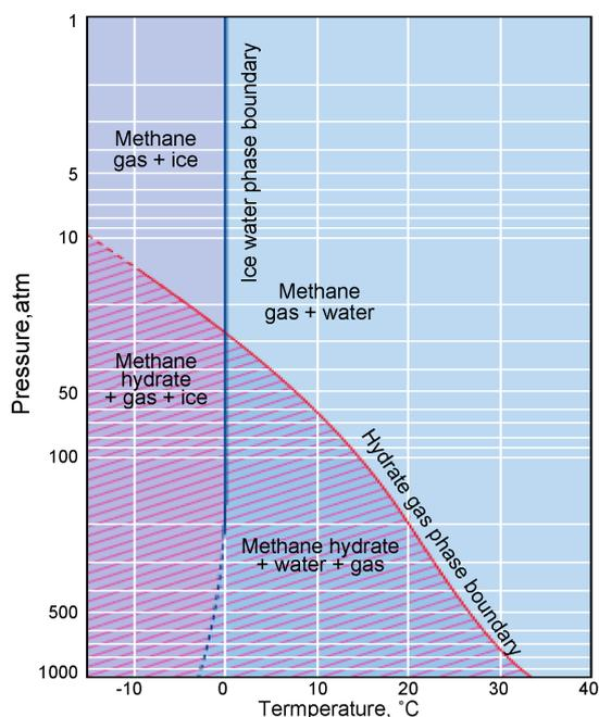
Figure 4. Phase diagram of gas hydrate stability [18].
