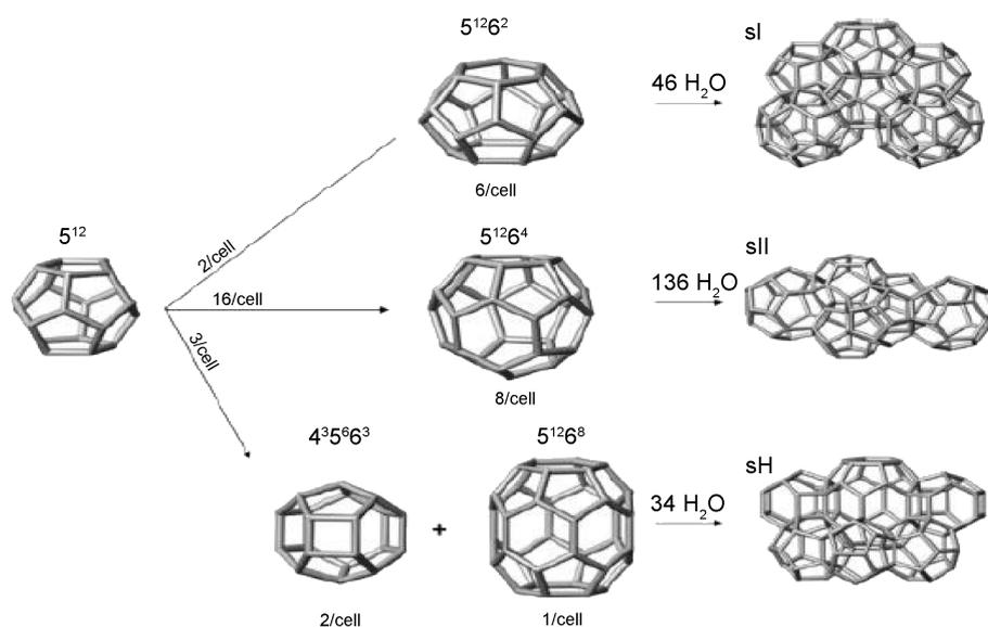
**Figure 5.** The structures of the classes of gas hydrate.
