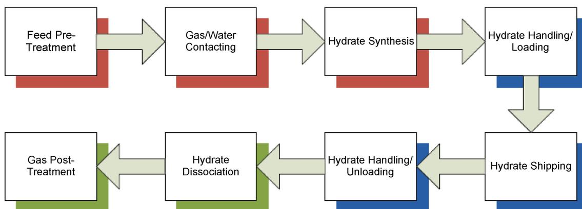
**Figure 6.** Schematic of a gas hydrate formation, transportation and dissociation system.
