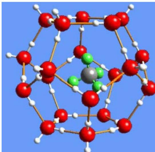
**Figure 3.** Cage-like structure of gas hydrate [18].
