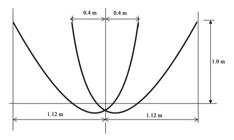
Figure 7. Reflector profile chosen for construction of the four wing CPC concentrator.
