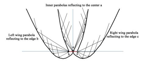
Figure 3. Alternative profile of compound parabolic concentrator with flat-base absorber.
