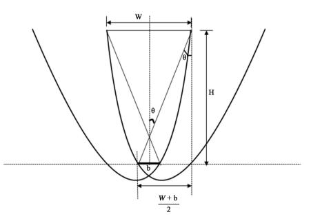
Figure 5. Dimensions of the internal wings of the regular CPC.
