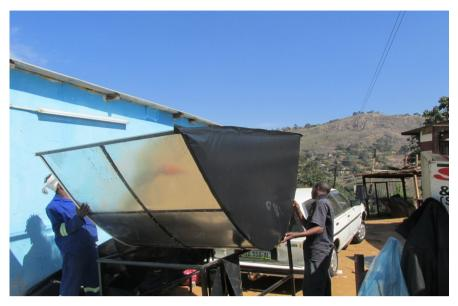
**Figure 11.** Side walls of the four wing CPC collectors wrapped with polyethylene sheets to preserve heat.
