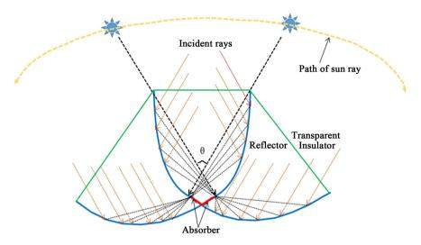
Figure 2. Profile sketch of a four wing compound parabolic collector with v-shaped absorber.
