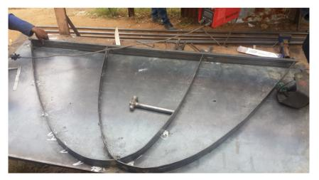
Figure 8. Constructing the four wing CPC profile on a sheet metal base.
