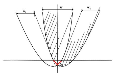
**Figure 6.** Additional aperture widths ( $W_E$ ) due to the added outer wings of the parabola.
