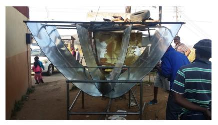
Figure 9. Construction of the wings, frame, absorber and reflector surfaces.
