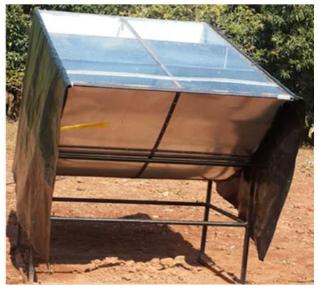
Figure 12. Completed installation of the four-wing CPC at the pilot trial site.
