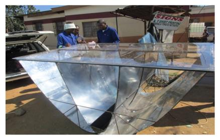
Figure 10. Top Perspex glass cover of 4 mm thickness fitted for insulation and preservation of heat.
