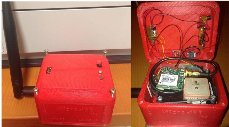
**Figure 10.** Wireless Micro intelligent Black Box (Micro-iBB).
