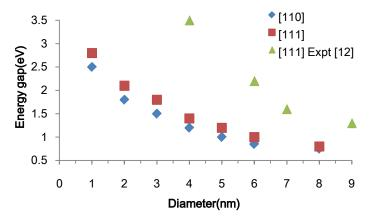
**Figure 2.** Band gap of the SiNWs versus the cross-sectional diameter, blue dots is for [110], brown for [111], and green for experimental data taken from reference [17] for [111].
