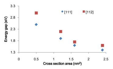
**Figure 3.** Band gap of the SiNWs versus the cross-sectional area, blue dots is for [111], brown for [112].
