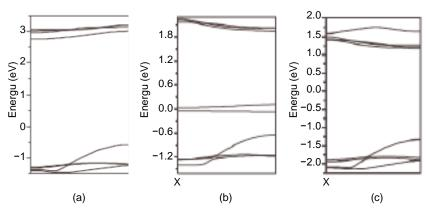
Figure 4. Diagram for electronic band structure (a) SiNW, (b) SiNW with N doped, (c) SiNW with -OH group.
