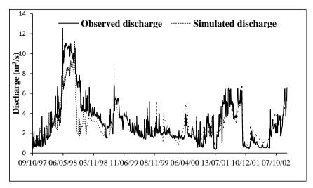
**Figure 3.** Observed and simulated daily discharge for the Murchison Bay catchment during calibration (1997-2002).
