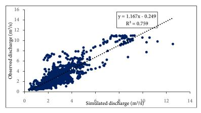
**Figure 5.** Scatter plot of observed and simulated discharge for the calibration period (1997-2002).
