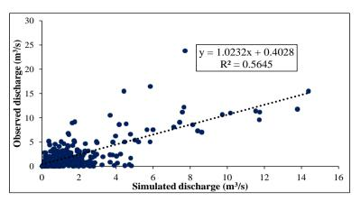
**Figure 6.** Scatter plot of observed and simulated discharge for the validation period (2004-2007).
