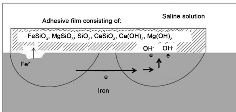
**Figure 11.** Proposed barrier mechanisms to silicate in the saline solution.
