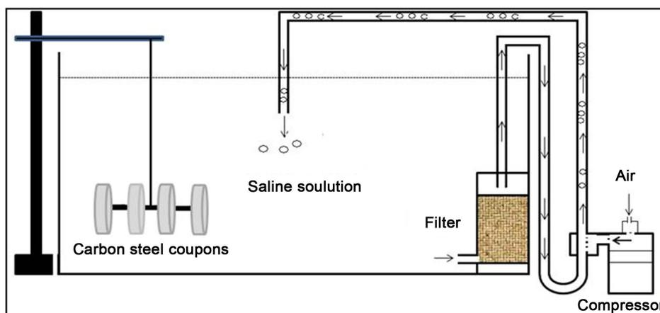
**Figure 2.** Assay carbon steel immersed in seawater.
