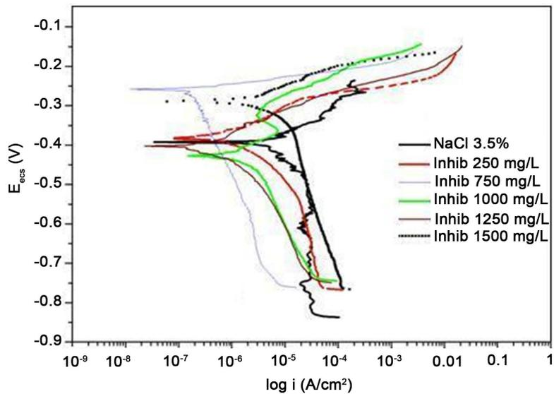
**Figure 9.** Anodic and cathodic Tafel polarization curves for carbon steel in the absence and presence of various concentrations of the corrosion inhibitor to the base sodium silicate.
