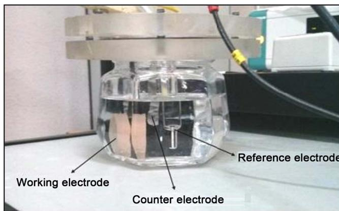
**Figure 3.** Conventional polarization cell.
