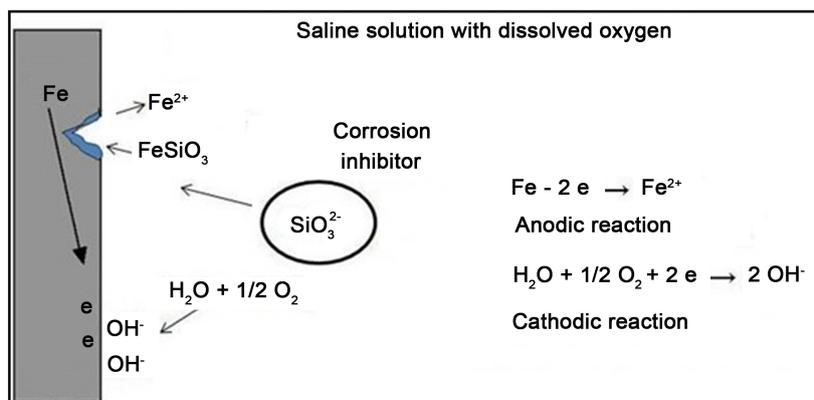
**Figure 10.** Silicate formation on a metal surface in a saline solution with dissolved oxygen.
