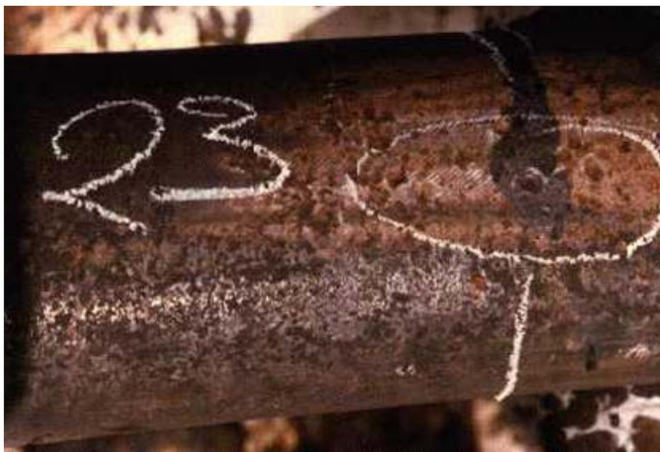
**Figure 1.** Pitting in a drill pipe.
