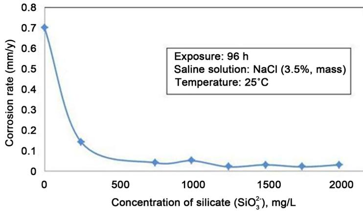
**Figure 7.** Rate of corrosion of the carbon steel coupon in the saline solution with the silicate corrosion inhibitor, 96 h.
