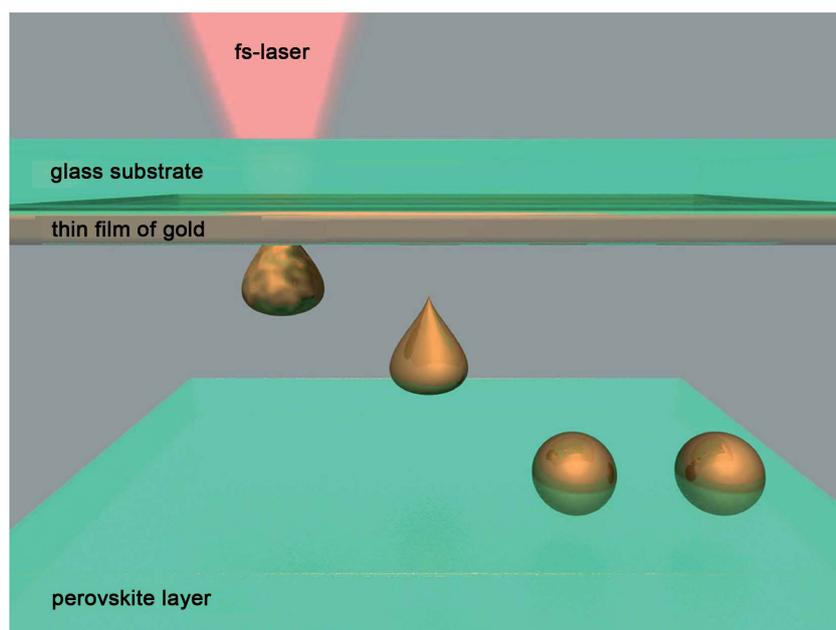
**Figure 6.** A sketch of the laser-induced forward transfer of gold nanoparticles into perovskite.
