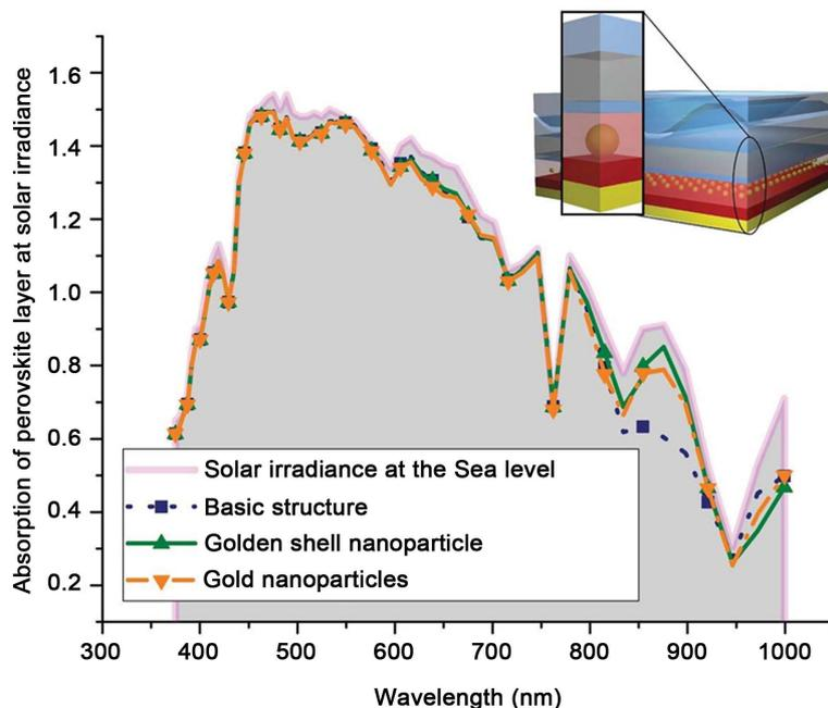
**Figure 5.** Absorption in the perovskite layer for several variants of our solar cell (basic structure, the structure enhanced by solid nanospheres, and that enhanced by nanoshells) taking into account the solar irradiance spectrum.
