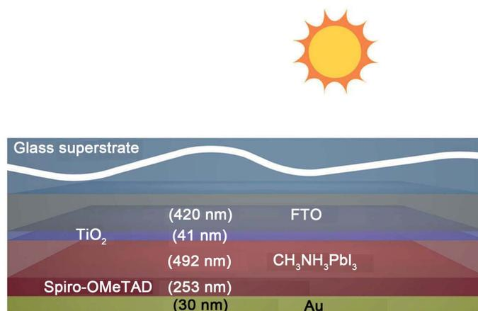
**Figure 1.** Schematics of the practical heterojunction configuration of a high-efficiency perovskite-based solar cell in accordance to [7]. The anti-reflecting coating on top of the superstrate is not shown.
