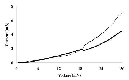
**Figure 3.** Plot of current vs. voltage for electroxidation of ethanol for SDS modified (thin line) and SDS unmodified (thick line) iron deposited graphite electrode.
