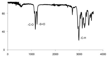
Figure 1. FTIR spectrum of layer removed from SDS modified graphite electrode.
