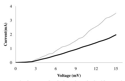
**Figure 2.** Plot of current vs. voltage for electroxidation of methanol for SDS modified (thin line) and SDS unmodified (thick line) iron deposited graphite electrode.
