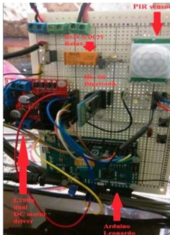
Figure 4. Receiving and control circuit.
