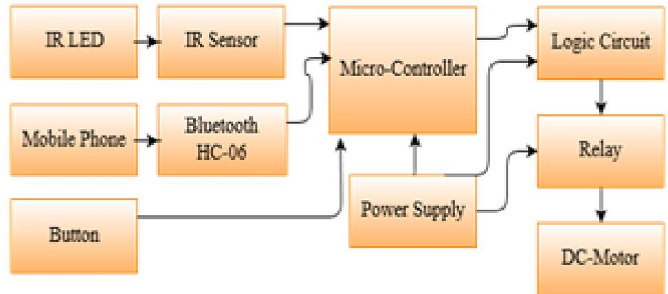
**Figure 1.** The block diagram of an automatic door.
