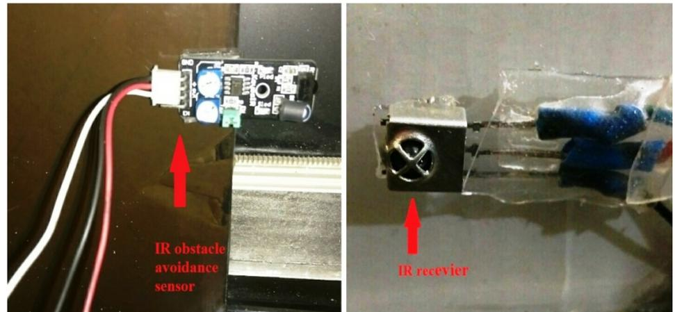
Figure 3. IR sender and IR avoidance.
