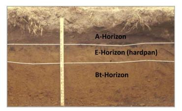
Figure 1. A typical soil profile of the coastal plain in the southern USA.
