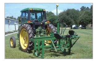
Figure 3. The tractor mounted soil compaction measurement system.
