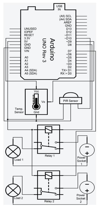
**Figure 1.** Schematics of the connection that controls an electric appliance (*load*) using a relay and Arduino Uno.
